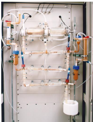
Figure 1. TNO gastro-Intestinal Model simulating the stomach and small intestine (TIM-1).
